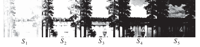
Fig. 4. Images given by truncating of the original image histogram at points \lambda_i correspondent to cumulative histogram slices S_i for \Lambda = 5
