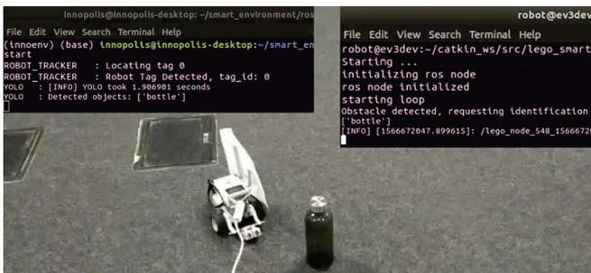
Fig. 9. Smart Space’s node identifies the robot location and obstacles around the robot, and sends the list of obstacles detected back to the robot
