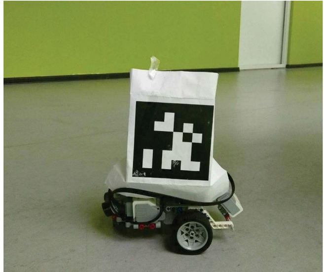
Fig. 6. The Lego Mindstorm EV3 robot with the attached AprilTag label
