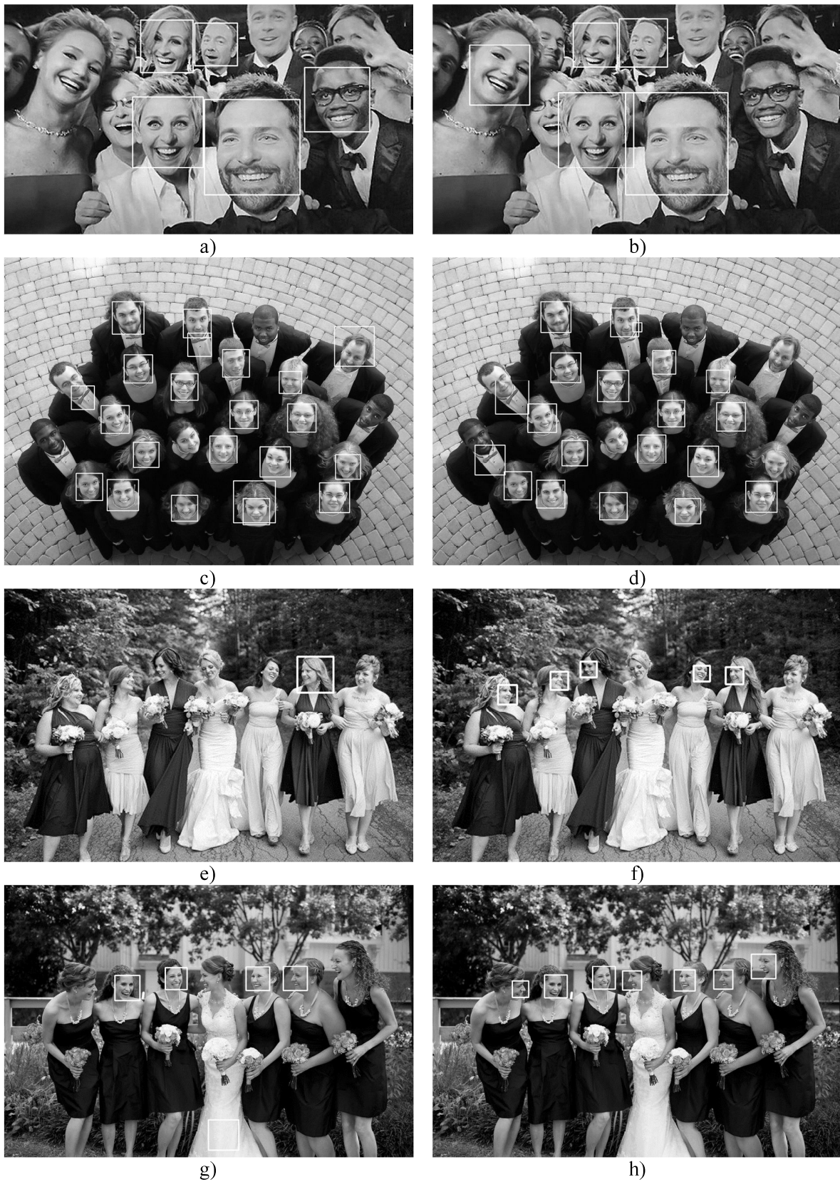
Fig. 5. Visual examples of face detection algorithm quality: a), c), e), g) Viola-Jones algorithm; b), d), f), h) CEDT approach
