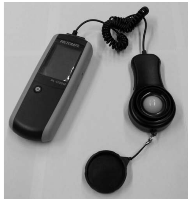
Fig. 19. Voltcraft PL-110SM solar radiation measurement instrument
