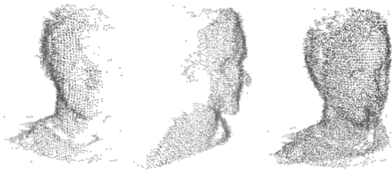
Fig. 10. Combining source point clouds into a complete model of the object using the set of proposed algorithms
