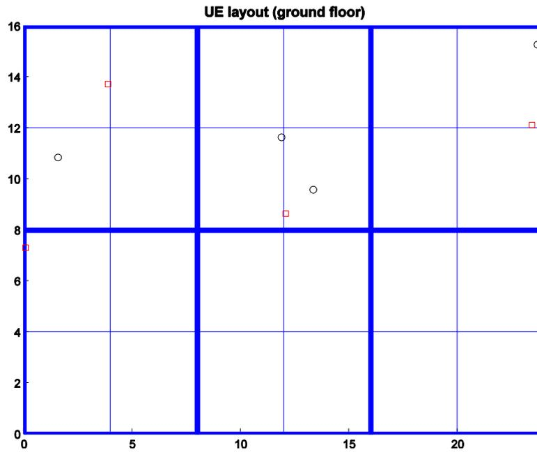
Fig. 3. Example of a  $3 \times 2$  grid floor layout belonging to a multi-floor apartments block
