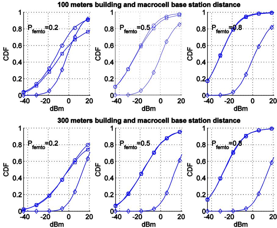
Fig. 5. CDFs of EUE transmission power in multi-floor apartment block. Line with circle denotes both MBS and HBSs are granted access to EUE. Line with square denotes only HBSs access. Line with diamond denotes only MBS access
