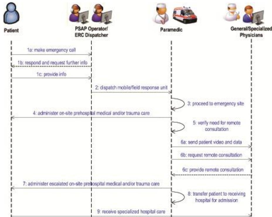
Fig. 1. Use case description sequence diagram
