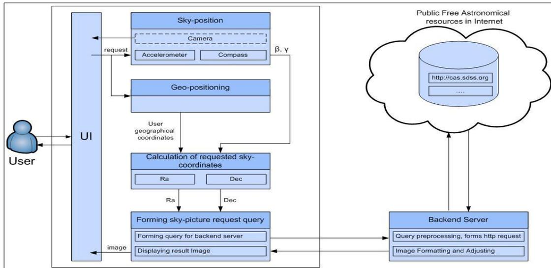
Figure 1: The Virtual Telescope service architecture for mobile devices.
