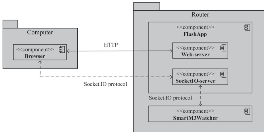
Fig. 2. Smart-M3 Control Panel system architecture
