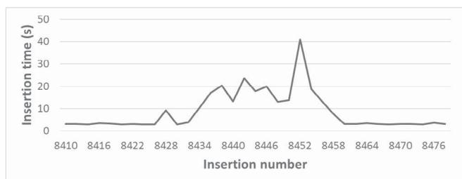
Fig. 9. Example of router slowdown during insertion test
