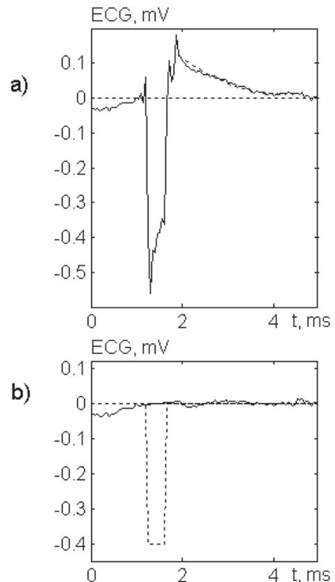
Fig. 2. Illustration of the spike detection algorithm and further signal correction: a) a fragment of raw signal containing a pacemaker spike (solid line) and polynomial curve used for the polarization jump compensation (descending dotted line); b) the same signal fragment after the pulse deleting and the jump compensation (solid line); dotted line shows the detected pulse restored with the use of its parameters.
