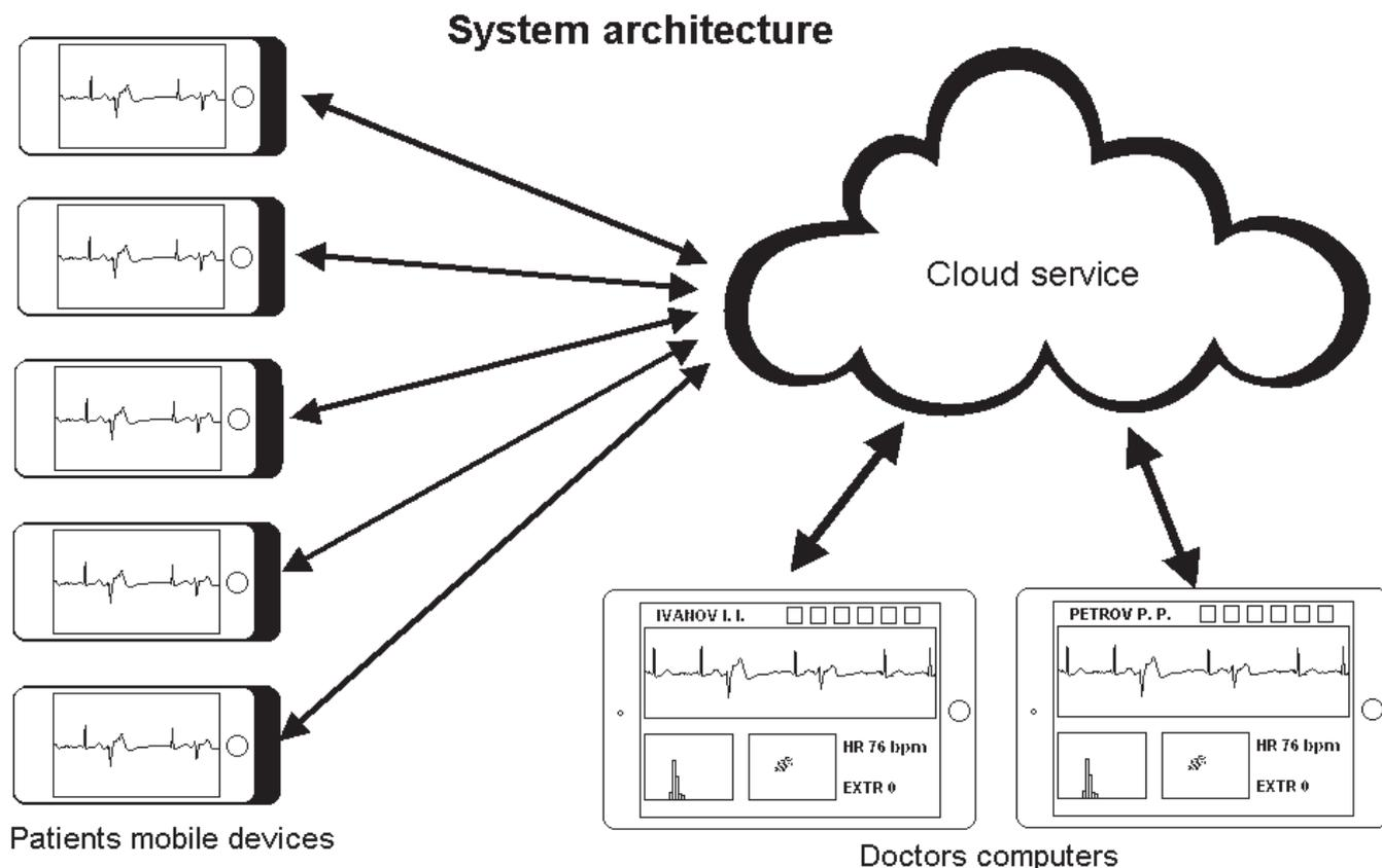
Fig. 1. Common architecture of the mobile cardiac monitoring system. Patients use their personal smartphone based ECG acquisition devices for the ECG registration and transfer to the cloud service via mobile phone connection and Internet. Doctors get access to the patients data with the use of their smartphones or computers.
