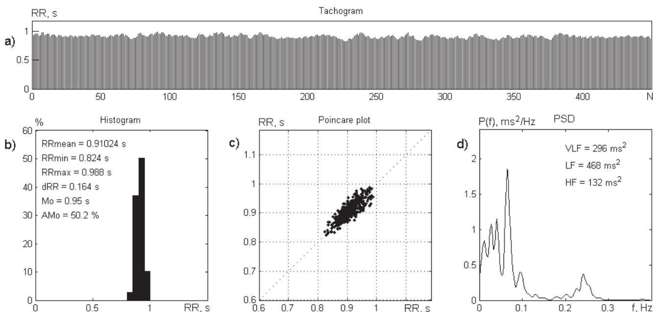
Fig. 5. The forms of cardiac rhythm graphical representation used in the system: a) RR-intervals tachogram; b) RR-intervals histogram and time domain HRV parameters; c) Poincare plot of RR-intervals; d) heart rhythm power spectral density plot and frequency-domain HRV parameters
