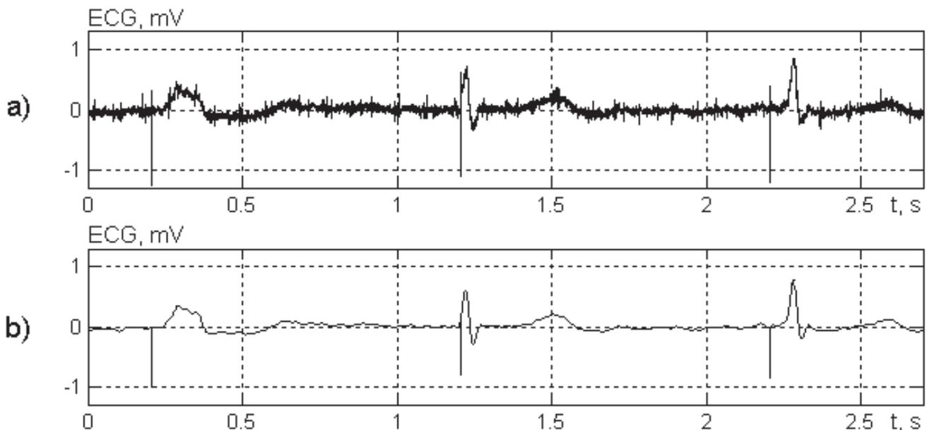
Fig. 3. Reconstruction of the detected pacemaker spikes for the ECG display. Raw wide-range ECG signal with sampling frequency 20000 Hz in which pacemaker pulses take place (upper plot) and the same signal after the correction of the segments containing spikes, smoothing, decimation and restoring of the detected pulses (lower plot).
