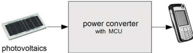
Fig. 6. Structure 2: Mobile phone as passive device
