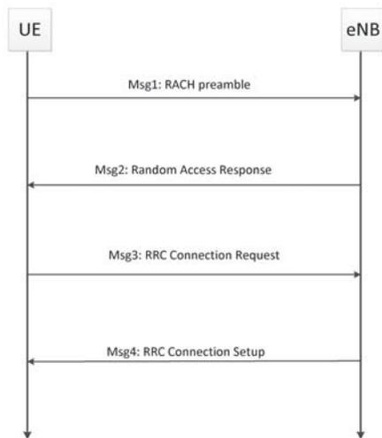
Fig. 4. RA procedure signaling.
