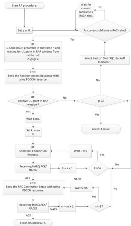
Fig. 5. Algorithm of RA procedure.
