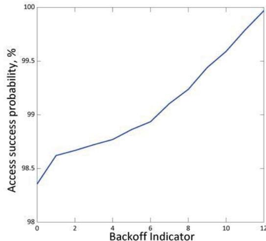
Fig. 7. Dependence of the access success probability on the value of backoff indicator.
