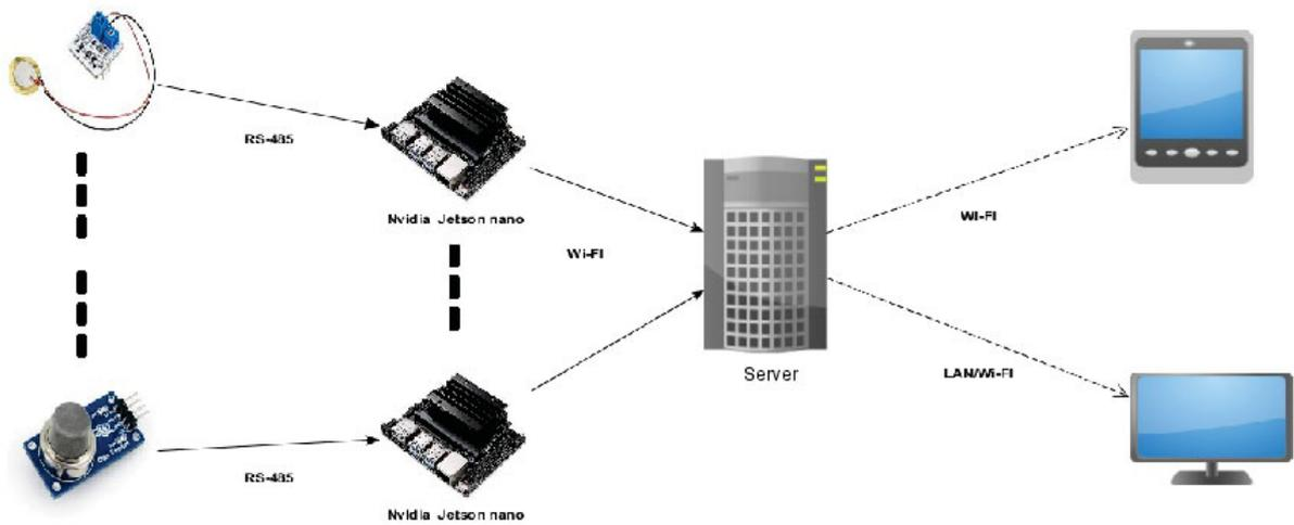
Fig. 2. Fault detection service: architecture
