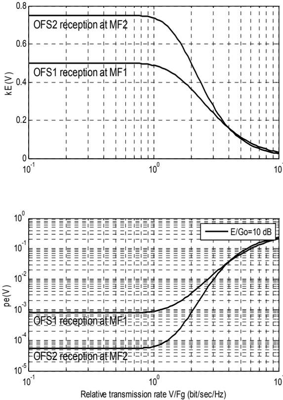
Fig. 6. PTR and average error probability dependences on bit rate
