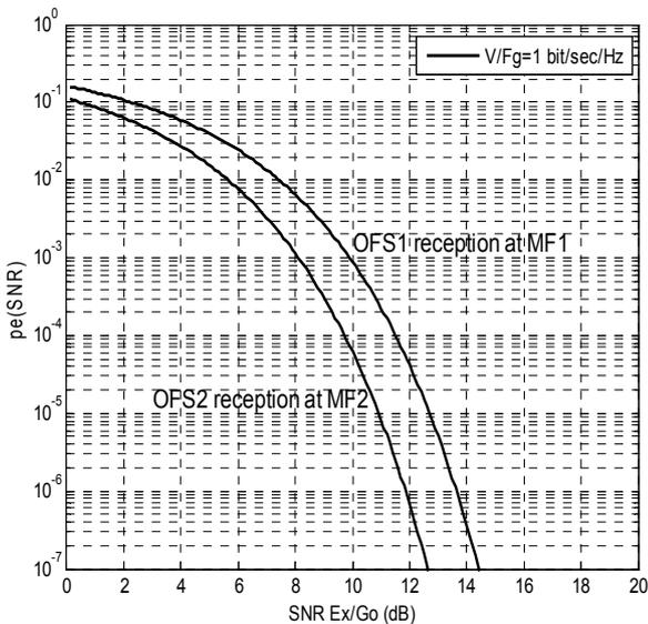
Fig. 7. Average error probability dependences on the signal-to-noise ratio
