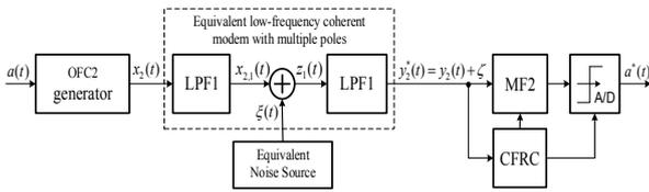
Fig. 4. Low-frequency equivalent of optimal modem with multiple poles
