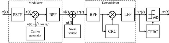
Fig. 1. Model of data transmission system with coherent modem
