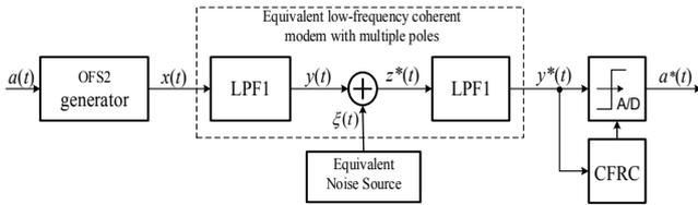
Fig. 2. Coherent modem's low-frequency equivalent model
