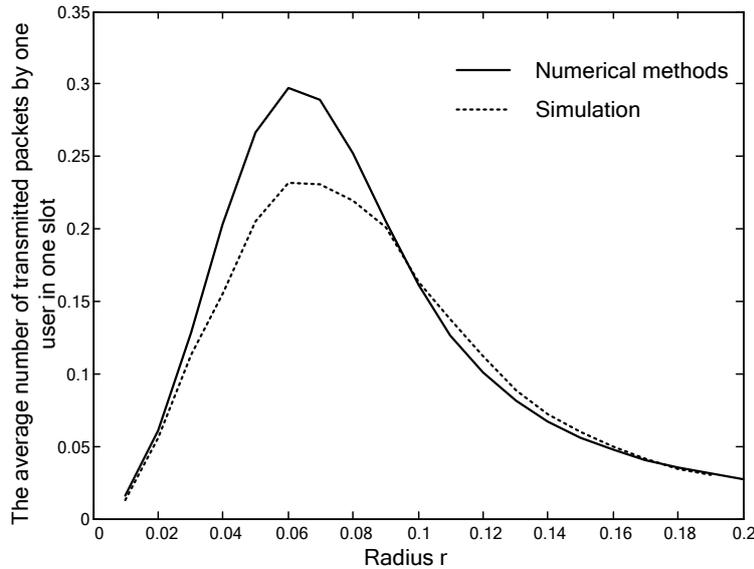
Fig. 3. The dependence of average number transmitted packets in the slot by one of the users on radius  $r$
