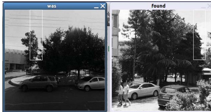
Fig. 1. False positive result of OpenCV::matchTemplate method. Fragments similarity K = 80.36\% .
