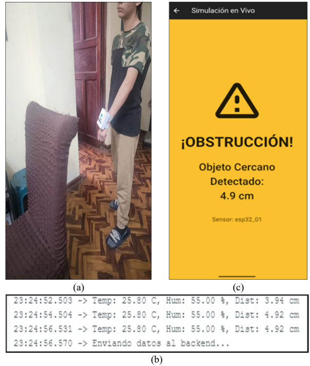
Fig. 13. Results of scenario 2: Visually impaired user near an obstacle(a), console results by IoT device (b) and results in the mobile app (c)
