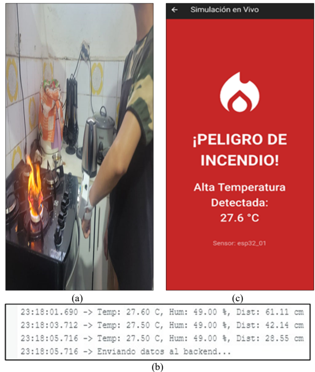
Fig. 14. Results of scenario 3: Visually impaired user near fire (a), console results by IoT device (b) and results in the mobile app (c)
