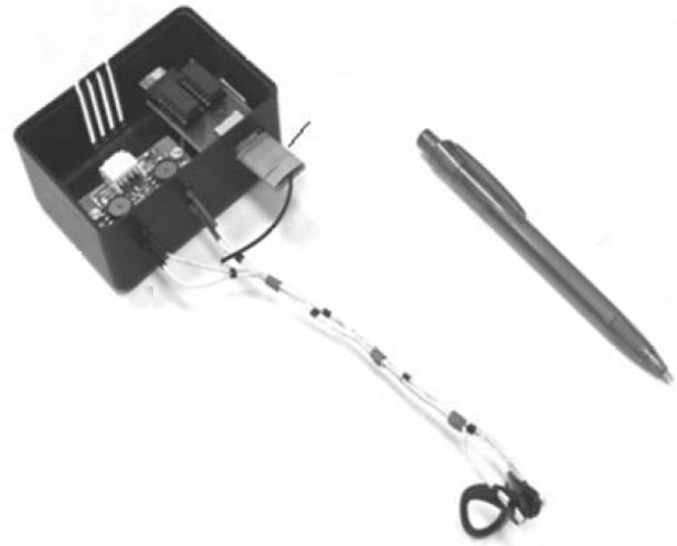
Fig. 1. A prototype of the device using two pressure sensors, with the ends of the outlet tubes attached to a clip
