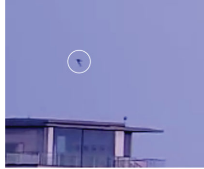
Fig. 4. Illustration of a minimum-size training object (5×5 pixels), representing the lower bound of detectable targets
