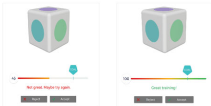
Fig. 2. Training interface (EmotivBCI). The reference box with 8-second timer per training to execute the command “upward”, “downward”, “neutral”. Training results: goal not reached (left), goal reached (right)
