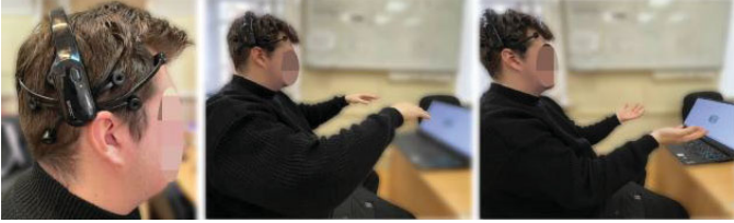
Fig. 1. Device setup (Emotiv Epoc X). Placement of electrodes on the participant's head (left), downward movement (middle), upward movement (right)
