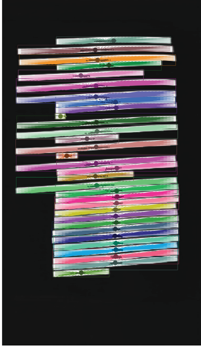
Fig. 5. Instance segmentation mechanism. Black and white background reflects the visibility p of pixels, lines show the offset vectors (d_x, d_y) , dark dots show predicted box centers for different pixels
