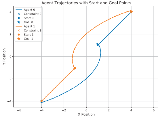
Fig. 1. Two-agent crossing scenario: planned trajectories. Both robots reach their goals without collisions
