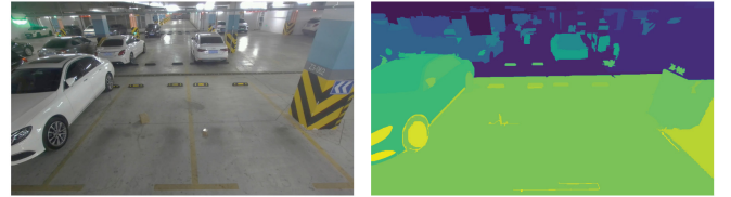
Fig. 3. Original test image (left) and its graph segmentation visualized as the colormap (right) using Pegtop soft light blending with an inverse copy of the image
