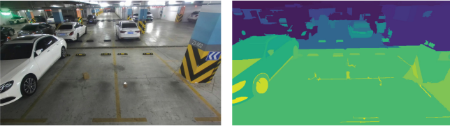
Fig. 2. Original test image (left) and its graph segmentation with implemented color map (right) without pre-processing
