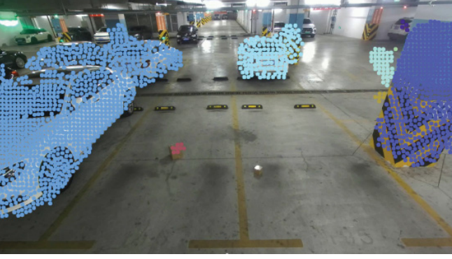
Fig. 12. The results of object segmentation by stereo image-based method with SLIC superpixel segmentation
