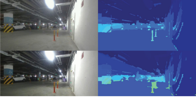
Fig. 4. Original images (left) and images with the results of their graph segmentation (right). The bottom images are before pre-processing, and the top image - after Pegtop soft light blending (with its inverse copy) applied to the bottom original image
