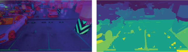
Fig. 5. Original test image after RGB to HSV color space conversion (left) and its graph segmentation visualized as the colormap (right)
