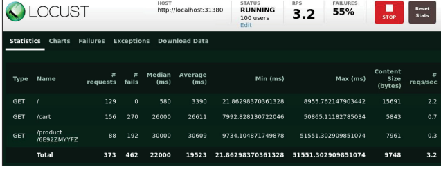
Fig. 7. Locust load testing statistics under delay fault
