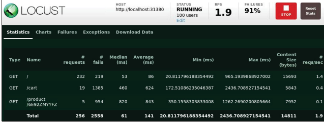
Fig. 8. Locust load testing statistics under abort fault
