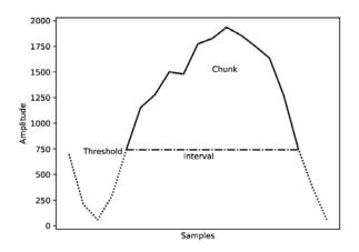
Fig.1. Wave as a part signal under investigation
