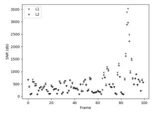
Fig.3. Compare optimal thresholds computed by full search and (5); sample frequency = 16 kHz, length of fragment = 512. L1 - full search for Trs with step = 20, L2 - linear regression
