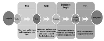
Fig. 2. Basic VUI pipeline
