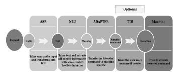
Fig. 5. Pipeline of proposed integration from request to execution
