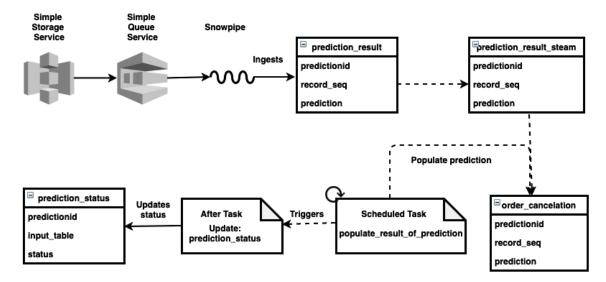
Fig. 5. Flow diagram of piping the data into Snowflake
