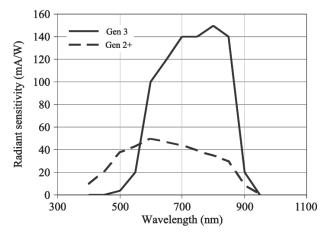
Fig. 2. Color sensitivity of night-vision devices of 2 and 3 generation
