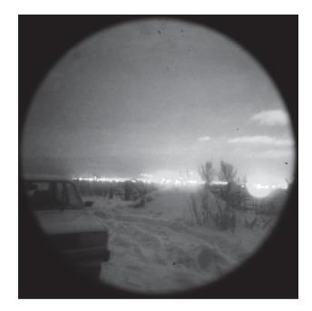
Fig. 1. Example of bloom effect in night vision device. The distance to light sources is about  $1.5 \mathrm{km}$
