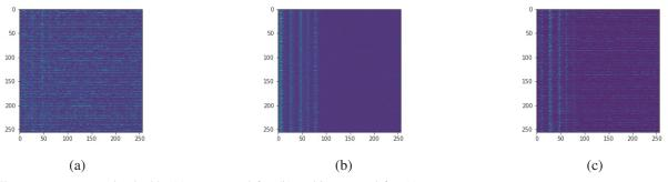
Fig. 1. The spectrogram examples: healthy (a), outer race defect (b), and inner race defect (c)
