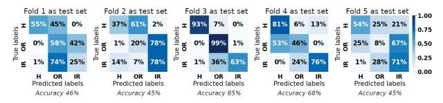
Fig. 10. The confusion matrices for 5 combinations of training and testing data normalized over the true conditions and averaged over 5 training trials
