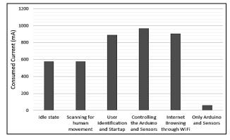
Fig. 15. The current consumption rate of various tasks & states
