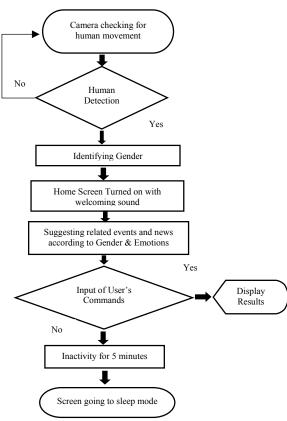
Fig. 2. Image Processing Flowchart
