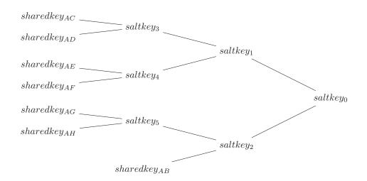
Fig. 2. Binary tree of saltkeys for seven friends  $B, C, \dots, H$  of A in Protocol 2.
