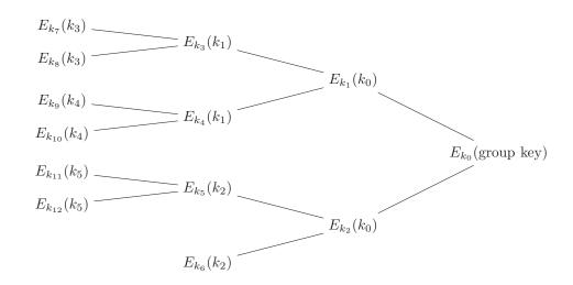
Fig. 1. Logical key hierarchy for seven members. Keys  $k_6, k_7, \ldots, k_{12}$  are distributed to the members With a personal key a member can decrypt another key and finally the group key as long as all the encrypted values are made available.
