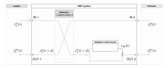
Fig. 1. Schematic representation of the adaptive metronome technique
