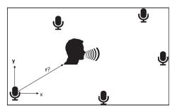
Fig. 1. Source localization with 5 single-channel microphones
