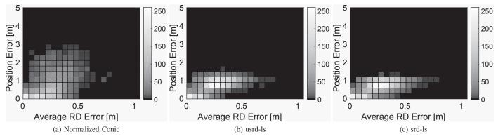
Fig. 5. Histogram of the average RD errors vs position errors
