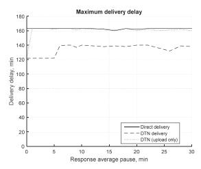
Fig. 17. Maximum delivery time with response-to-request message scheme depending on average response time (normally distributed random value) for all mobile operators available.
