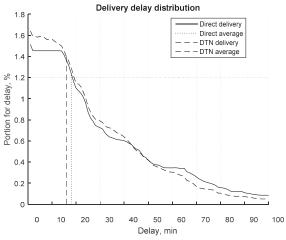
Fig. 14. Average delivery delay distribution with and without DTN (except immediate delivery with zero delay).
