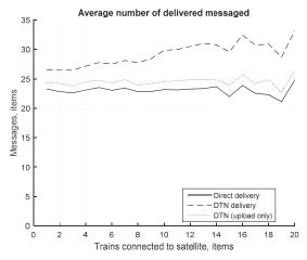
Fig. 21. Average number of delivered messages per train (only for the trains that are not connected to a satellite) depending on number of trains connected to satellites
