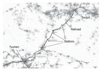
Fig. 13. Tyumen-Surgut railroad coverage map (for one mobile network carrier, MTS). Color intensity corresponds to quality of coverage.
