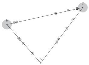
Fig. 7. An example of visualization of nodes location (denoted by letters), their connections, BS at some nodes (coverage is marked with big light gray circles around the nodes), objects (indicated by numbers) and TS coverage (small circles: normally without filling, gray while meeting TS, dark gray if connected to BS) at some time.
