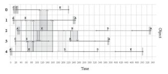
Fig. 8. An example of a visualization of the schedule for moving objects (objects are arranged vertically, the horizontal axis corresponds to the observation time). The horizontal lines correspond to the movement of the object between the control nodes. Vertical arrows visualize meetings and possible transmissions between objects.
