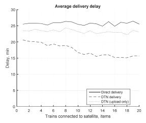
Fig. 22. Average delivery delay (only for the trains that are not connected to a satellite) depending on number of trains connected to satellites.
