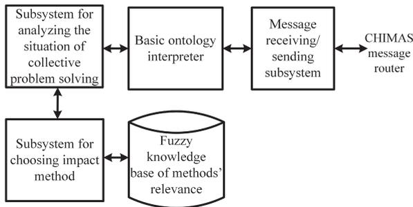
Fig. 7. The architecture of the agent-facilitator
