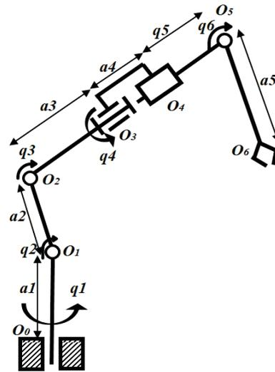
Fig. 1. The kinematic diagram of the manipulator
