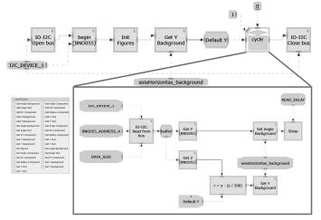
Fig. 3. VIPE program example with data coming from external sensor
