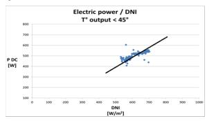
Fig. 5. Output power with respect to DNI in w/m<sup>2</sup> at 45 C
