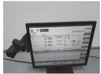
Fig. 5. Machine stand emulator: front view
