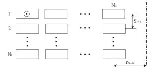
Fig. 9. Geometric parameters of inductors made on the printed circuit board
