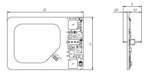
Fig. 1. General drawing of the wireless charging device. Receiving module
