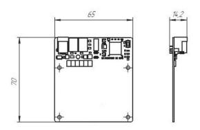
Fig. 2. General drawing of the wireless charging device. Transmitting module
