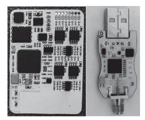
Fig. 6. Transmitting (left) and receiving (right) modules of the BTS
