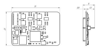
Fig. 5. General drawing of the implantable BTS. Transmitting module
