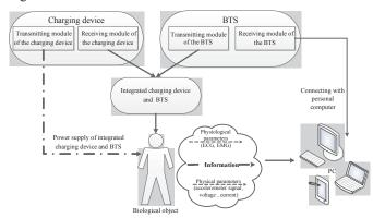
Fig. 8. Conceptual model of integration of wireless charging device and  $\ensuremath{\mathsf{BTS}}$
