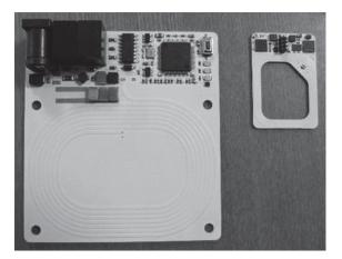
Fig. 3. Transmitting (left) and receiving (right) modules of the charging device
