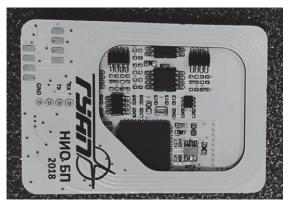
Fig. 7. Integrated charging device and BTS
