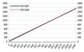
Fig. 14. Total amount of transmitted data in 4 channels with packets of up to 1500 bytes
