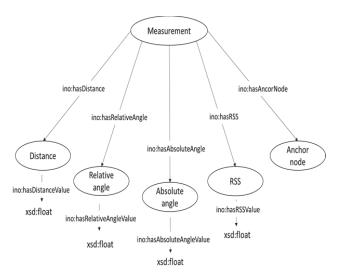
Fig. 5. Indoor Navigation Ontology fragment related to Measurement concept
