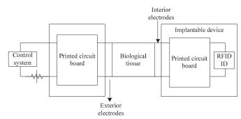
Fig. 3. Use of capacitor coupling for the implementation of a standard power and data exchange protocol
