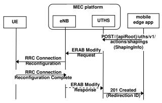
Fig.2. User traffic shaping by an authorized mobile edge application
