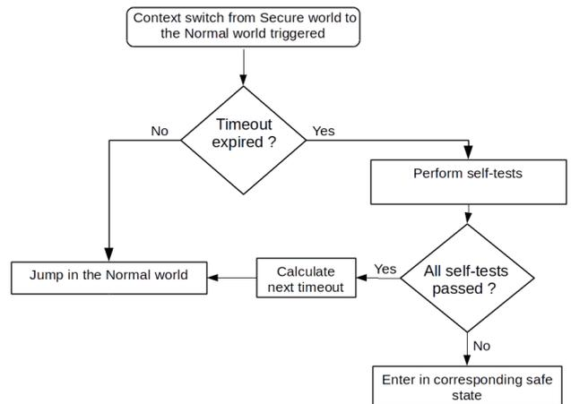
Fig. 6. Self-tests execution on Safety core
