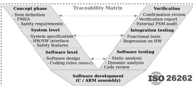
Fig. 1. V-Cycle ISO 26262 Road vehicles Functional Safety
