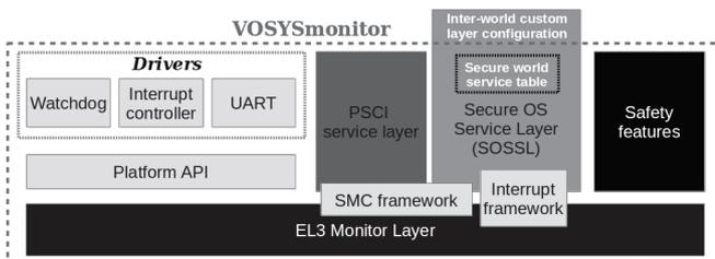
Fig. 4. VOSYSmonitor block diagram
