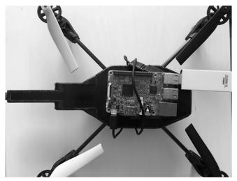
Fig. 5. UAV with Raspberry Pi and 4G modem
