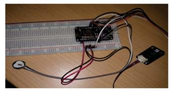
Fig. 2. Connections between sensors and Node MCU
