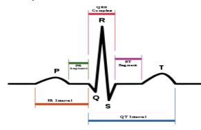
Fig. 6. Waves and Intervals on the ECG
