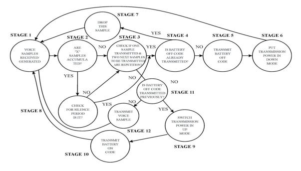
Fig. 4. State Transition Diagram for DITMC at mobile station
