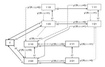
Fig. 6. The state diagram of the system with 2 VCs and buffer for 1 request
