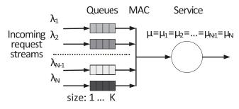
Fig. 2. Queue system of Output Virtual Channels SpaceFibre with MAC
