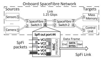
Fig. 1. Output Virtual Channels and MAC into out-port of SpaceFibre Switch
