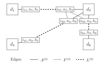
Fig. 4. Graph of the network layer of the sample network
