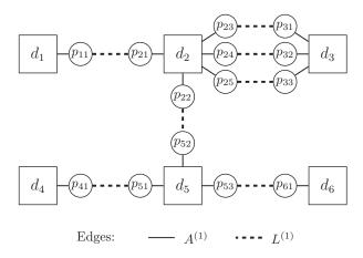
Fig. 2. Graph of the physical layer of the sample network
