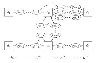
Fig. 3. Graph of the link layer of the sample network
