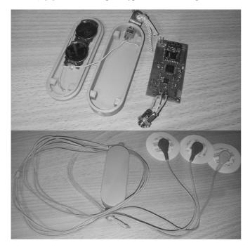
Fig. 2. ECG device prototype
